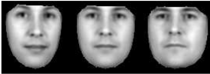
Figure 3.5: Example of the first mode of variation of the face using a statistical model of appearance. The parameter of \mathbf{c} corresponding to the largest eigenvalue varies from -3\sqrt{\lambda_1} to 3\sqrt{\lambda_1} .
